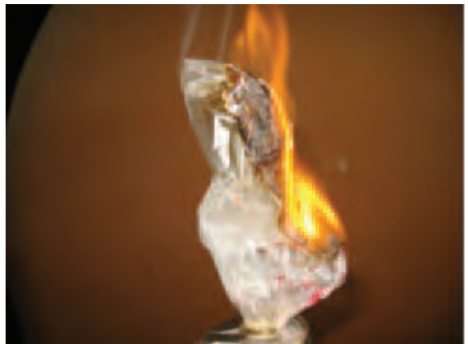
Figure 9 - Unlike plastics bags, true cellophane bags burn away without shrinkage
