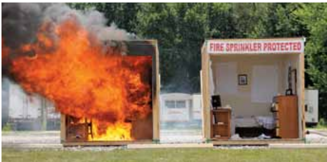
The sprinkler was activated less than a minute after the fire was ignited while the unprotected room burned out of control.
