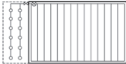
Figure 3: Exterior projection protected with two rows of sprinklers.
