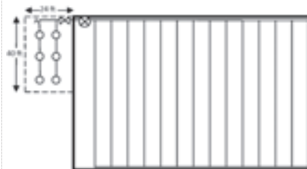
Figure 4: Small exterior projection protection by fire sprinklers.
