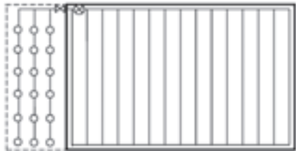
Figure 2(a): Exterior projection with multiple rows of sprinklers.
