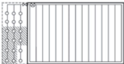
Figure 2(b): Remote area for light hazard exterior projection protected with a dry system.
