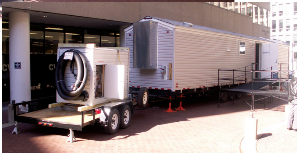
Sprinkler Manufactured Home with Pump & Tank Module
