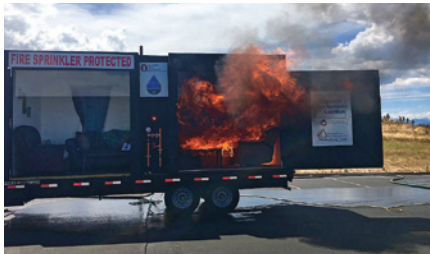
Flashover in less than three minutes, underscores NFSA's rallying cry of "Fire Sprinklers Buy Time. Time Buys Life." Pictured is the burn demo in Westminster, Colorado. A special thanks to NFSA member Western States Fire Protection Co. for sponsoring lunch & assisting with side-by-side. Teamwork at its best!
