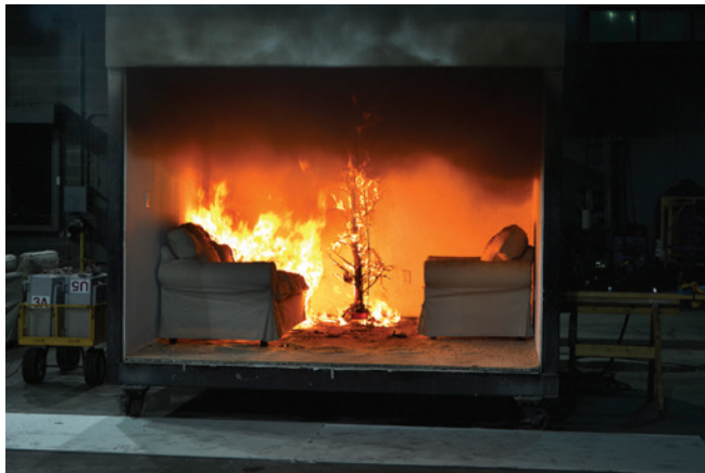
Figure 3 – test burn #3 – with sprinkler protection
