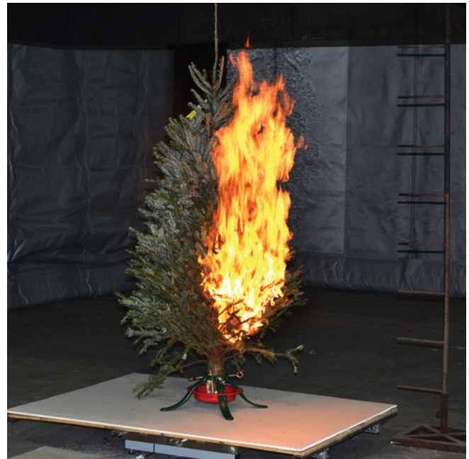
Figure 1 – burning tree under the calorimeter
