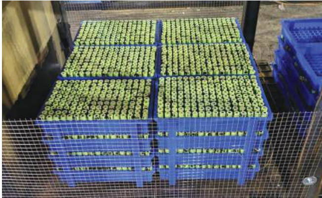
Figure 3: Trays Loaded with Lithium-Ion Batteries
